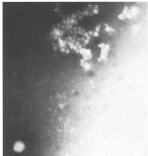
Fig. 3. Electron micrograph of poliovirus after incubation with aluminum. Large object is 79 nm bead.
